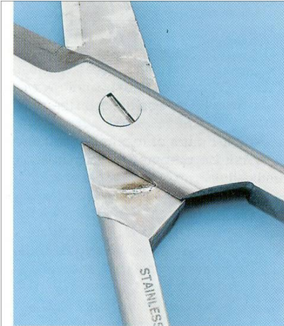
Fretting corrosion due to insufficient lubrication
