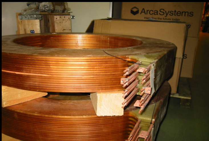
Magnet Coils, Preparation in the Factory
